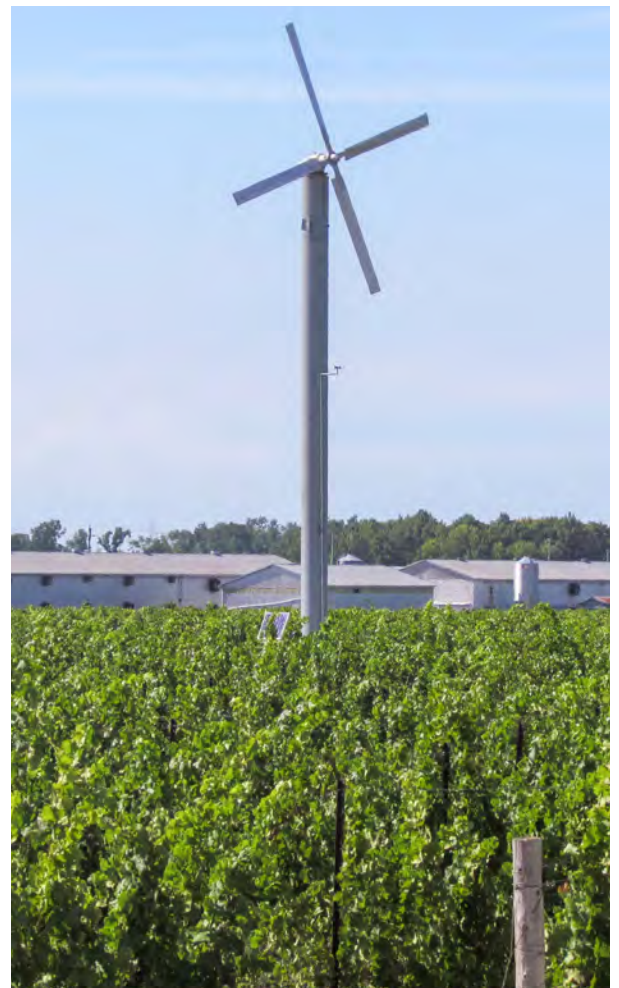
Figure 6.11 A wind machine being used to mix cool and warm air layers to prevent temperature inversions
