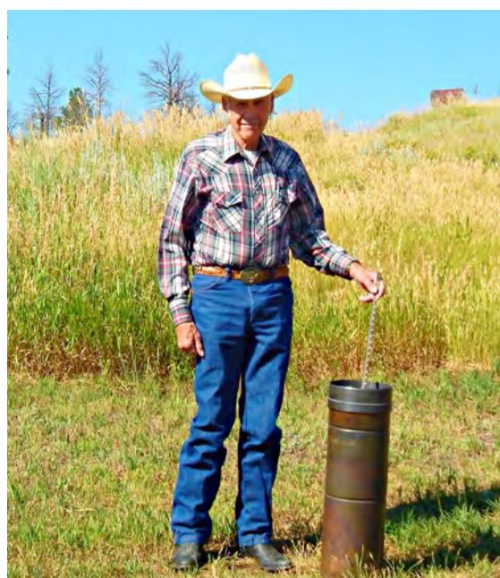
Figure 1. George Portwood stands next to the rain gauge on his property near RRS. This is a 'standard' National Weather Service (NWS) rain gauge. It consists of a funnel attached to a graduated cylinder (held by Mr. Portwood) that fits inside of the larger outside container, which is ~8 inches (20 cm) in diameter and 20 inches (50 cm) tall. The 8-inch gauge used in NWS Cooperative Weather Stations is of a standardized design used throughout the world for official rainfall measurements (National Weather Service Training Center, 2017). This standardization provides uniformity, continuity, and credibility of precipitation data. (Photo by B. Parker)
