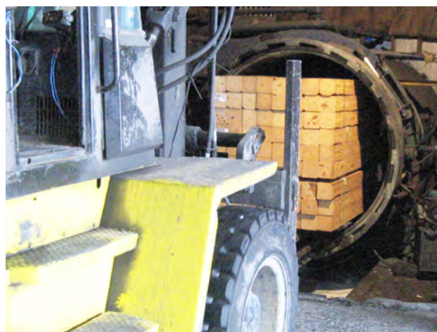
Figure 8-2. Using a forklift to push the charge into the cylinder for treatment.
