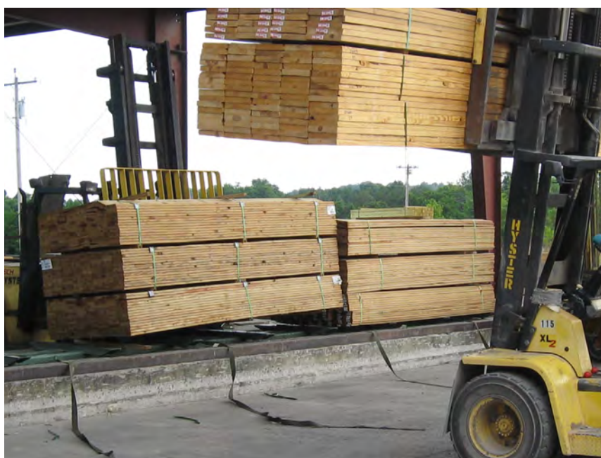
Figure 5-8. Transferring wood from storage yard to drip pad with two forklifts, one that stays on the pad and one that stays off of it.
