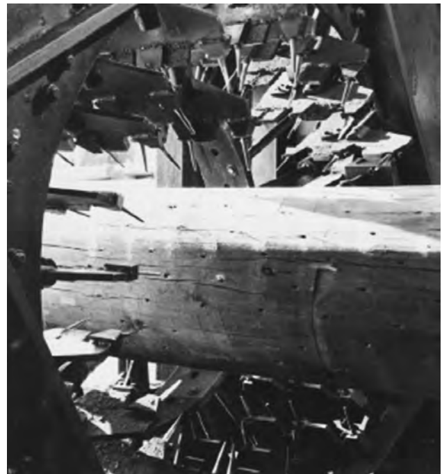
Figure 6-3. Incising permits better penetration of preservative. (Photo courtesy of USDA Forest Products Laboratory)
