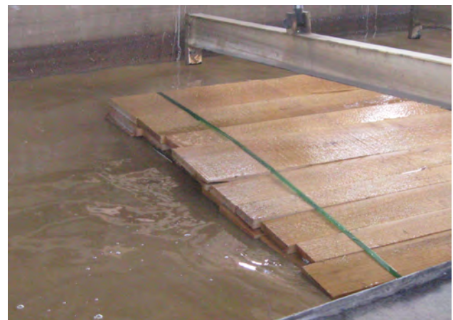
Figure 2-3. Rough-sawn lumber being dipped.
