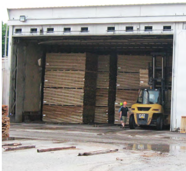
Figure 6-2. A kiln used to dry lumber at a sawmill.
