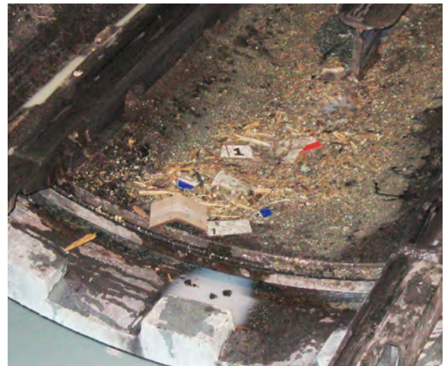
Figure 4-9. Examples of regulated wastes: preservative drippage from freshly treated wood (left) and process residuals, including sawdust, wood chips, and tags in a cylinder (right).
