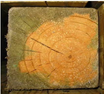
Figure 1-1. Effect of sapwood and heartwood on penetration by preservative in round utility pole (top) and sawn member (bottom). Photos: USDA Forest Products Laboratory
