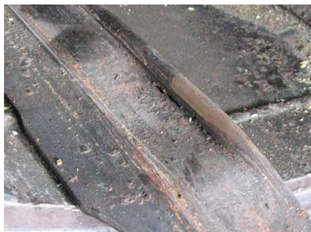
Figure 5-6. A welder certified in confined space entry would be needed to repair this broken weld on a track inside a cylinder.
