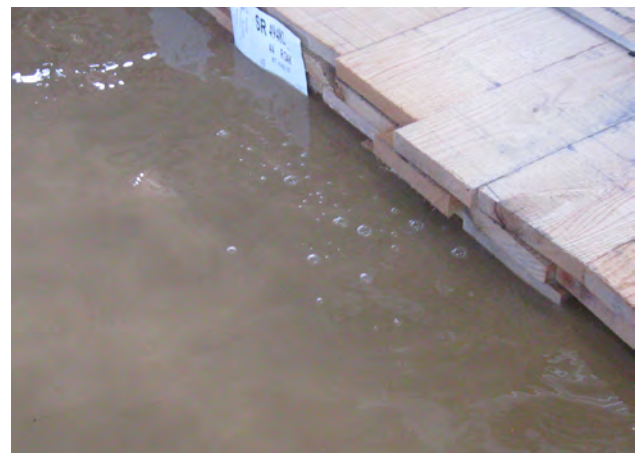
Figure 2-4. Air bubbles escaping from dipped wood.
