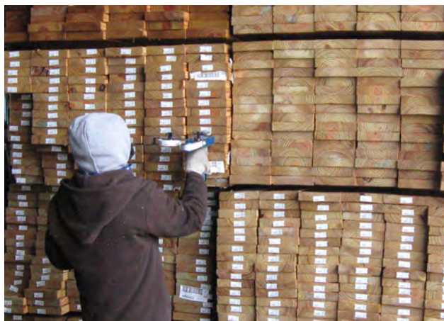
Figure 9-6. Tagging lumber after treatment.
