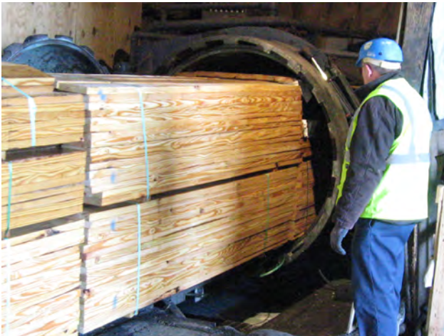
Figure 2-1. Loading a charge into the cylinder.
