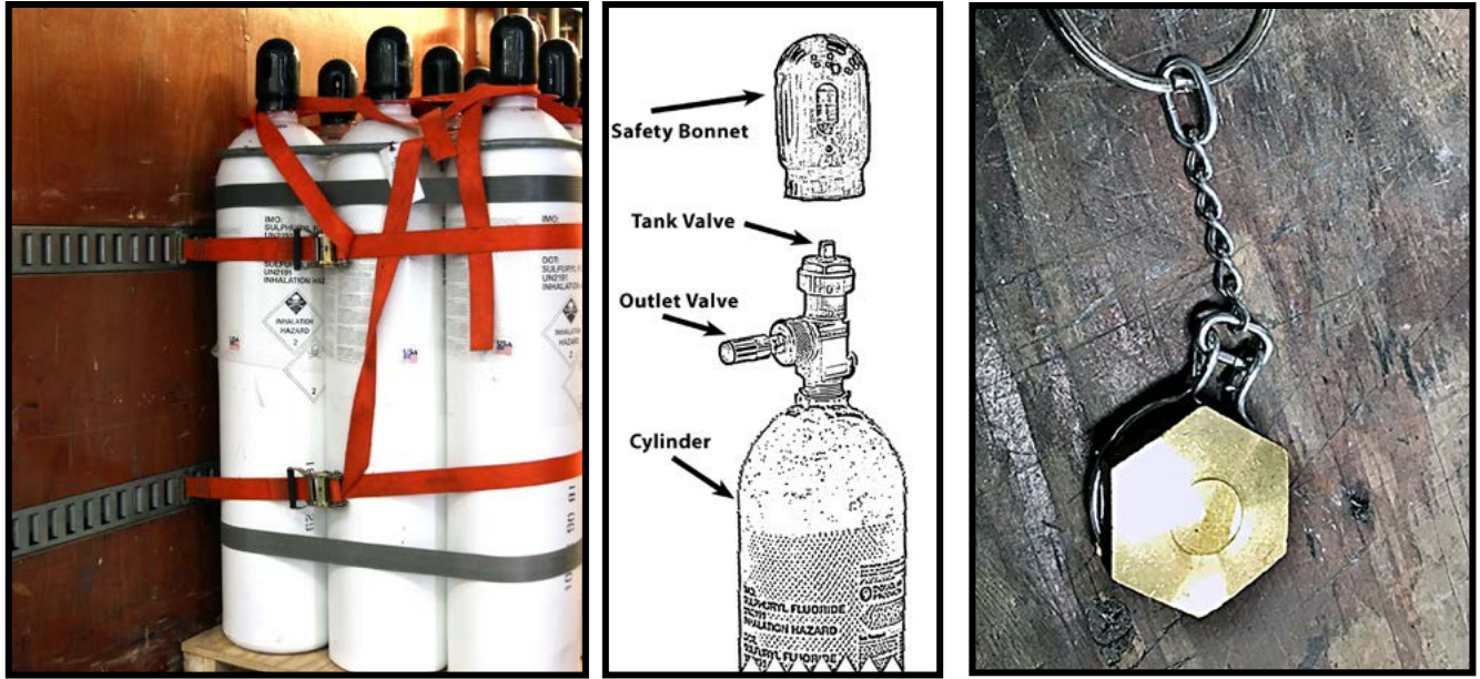
Figure 4: (Left) It is extremely important to secure fumigants so they will not move or get damaged during transport. Note that these cylinders are held fast with multiple ratchet straps. (Center) Always make sure the safety bonnets are screwed on over the valves except when in use. Fumigant cylinders may also come with covers over the outlet valves that also need to be in place until use. A valve cover is shown on the right. Photo and illustration credits: (left) © Garo Goodrow, Penn State; (center) diagram of cylinder based on © photos from Garo Goodrow, Penn State; (right) © Dale Dubberly.
