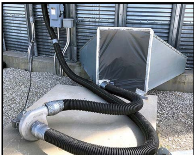
Figure 3: Using a recirculation system when fumigating a grain bin or other storage structure helps the quick and uniform penetration of phosphine throughout the commodity. In some cases, this could result in a reduced dosage. (Photo © Jeffrey Jones.)
