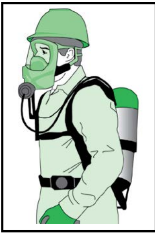
Figure 5: SCBAs supply clean air from a tank you carry. They have an alarm to warn you when the air supply is low. (Illustration © National Pesticide Applicator Certification Core Manual, NASDA).
