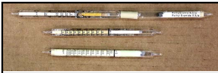
Figure 9: (Top) A worker checks for leaks of phosphine gas from a grain bin using a detector tube. (Bottom) Glass detector tubes are “fumigant specific,” meaning you need specific tubes to measure each type of fumigant you use. (Photo credits: (top) © Betsy Danielson, Iowa State University Extension and Outreach; (bottom) © Garo Goodrow, Penn State).
