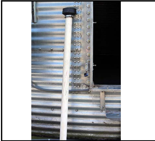
Figure 3: You can buy commercially made phosphine probes or make them from electrical conduit, plastic pipe, or tubing like the one pictured above. (Photo © Garo Goodrow, Penn State).
