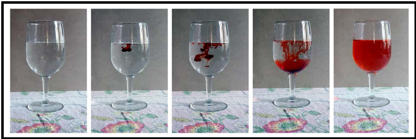
Figure 3: Diffuse (verb): to cause a gas or liquid to spread through or into a surrounding substance by mixing with it. Diffusion (noun): a process by which there is a net flow of matter from a region of high concentration to a region of low concentration resulting from random motion of molecules. The pictures above demonstrate diffusion using food coloring and water. The same principle applies to how a fumigant diffuses in air. (Illustration © UW-Madison Pesticide Applicator Training Program). (Illustration © UW-Madison Pesticide Applicator Training Program).
