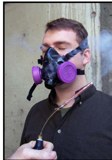
Figure 7: During a fit test, a user might be challenged with an irritating smoke or smell, such as a banana odor. If they can smell it, their respirator does not fit correctly. (Photo © Pacific Northwest Agricultural Safety and Health Center).
