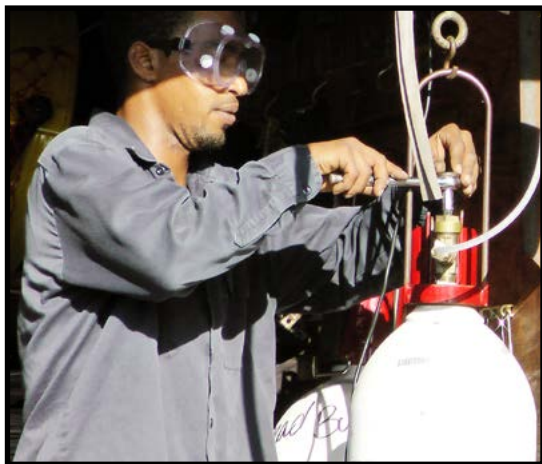
Figure 1: When releasing fumigant from a cylinder, wear eye protection and make sure that the hose discharges away from you. (Photo © Betsy Danielson, Iowa State University Extension and Outreach).
