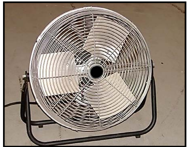
Figure 7: Fans are useful for aerating after a fumigation. Remember to use non-sparking fans to minimize the risk of fire. (Photo © Cardinal Products).
