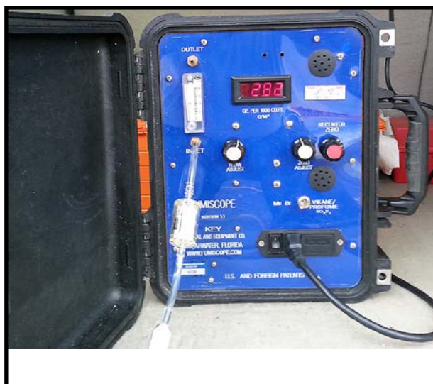
Figure 5: Monitoring for efficacy of fumigation is important to make sure the process is successful. Pictured above is one type of monitoring device, a fumiscope, which is generally used to measure methyl bromide or sulfuryl fluoride. (Photo © Carl Schnabel).
