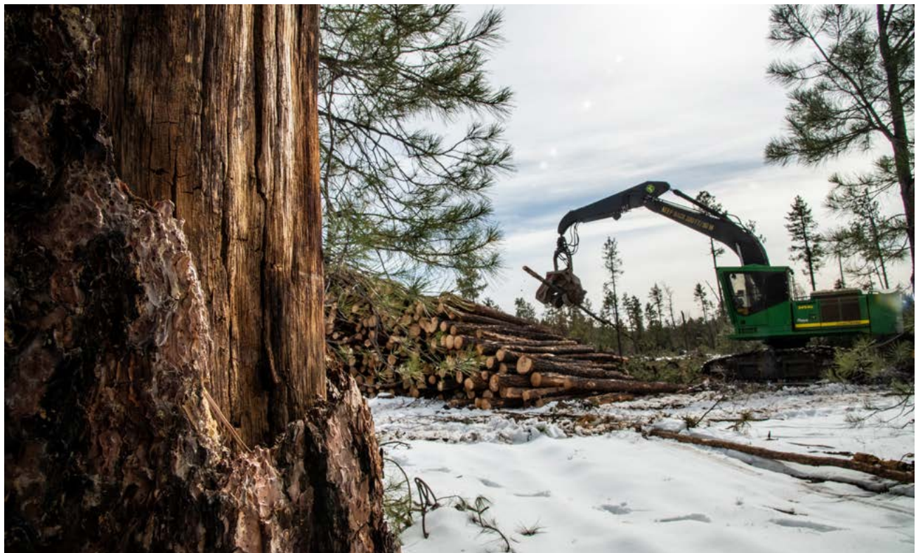
A harvester shoots a tree through removing its branches in seconds, then the bare tree trunk is cut to the desired length for sale. Kaibab National Forest, Arizona, December 4, 2018. (© USDA Forest Service, Lance Cheung)
