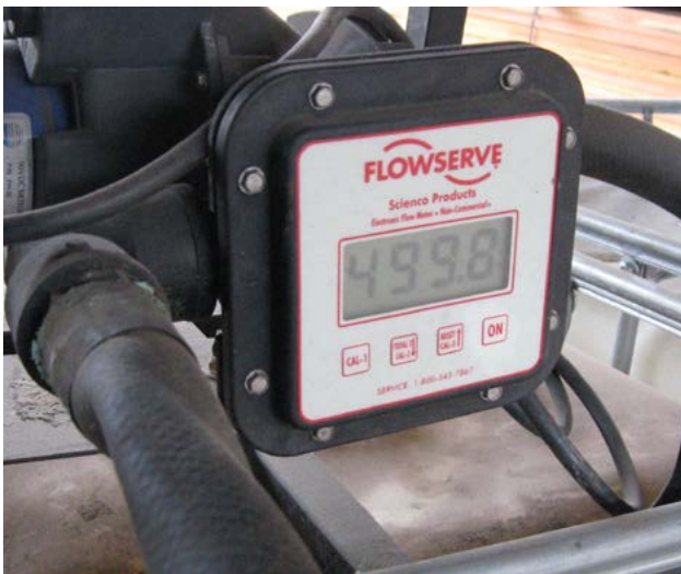
Figure 7-1. Tote flow meter
