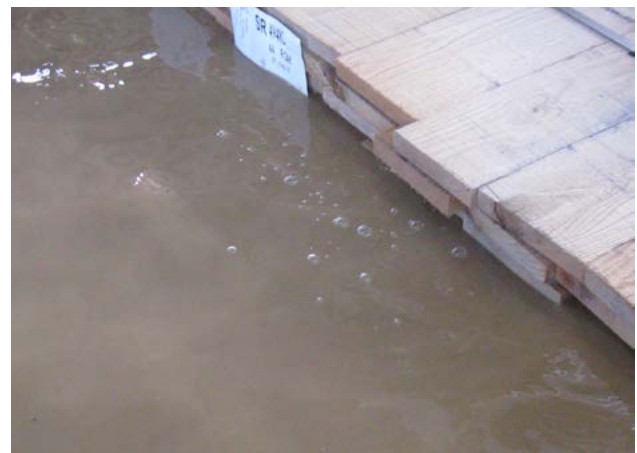
Figure 2-4. Air bubbles escaping from dipped wood.
