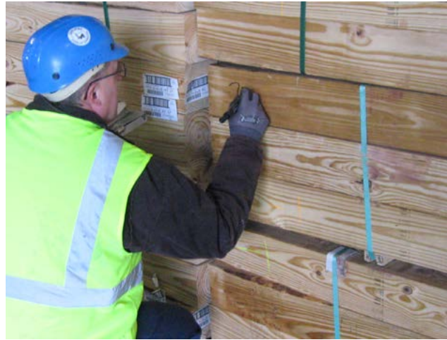
Figure 6-5. Marking wood with charge number prior to pressure treatment.
