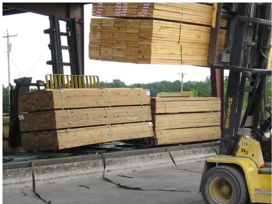
Figure 5-8. Transferring wood from storage yard to drip pad with two forklifts, one that stays on the pad and one that stays off of it.
