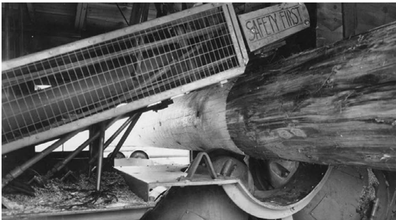
Figure 6-1. Machine peeling of poles. Here, the outer bark has been removed by hand and the inner bark is being peeled by machine. (Photo courtesy of USDA Forest Products Laboratory)
