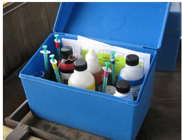
Figure 7-2. Kit for analyzing dip treatment solutions for preservative concentration.
