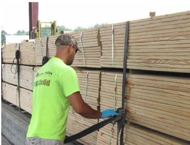
Figure 8-1. The charge is strapped to trams to keep it in place during treatment.
