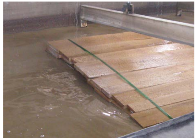
Figure 2-3. Rough-sawn lumber being dipped.
