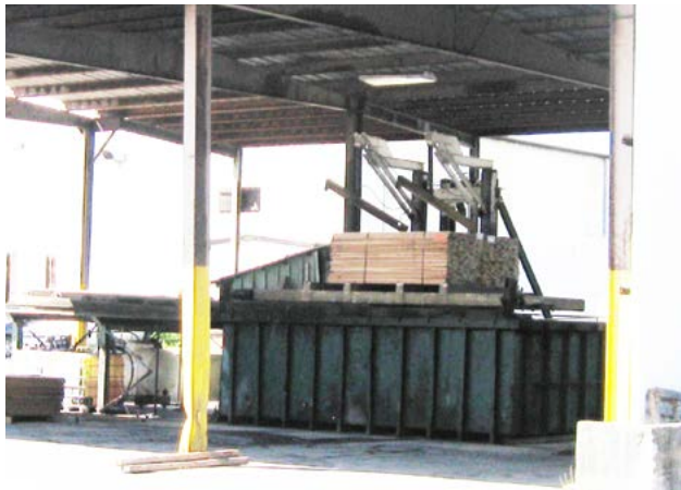
Figure 4-7. Wood loaded onto dip tank platform
