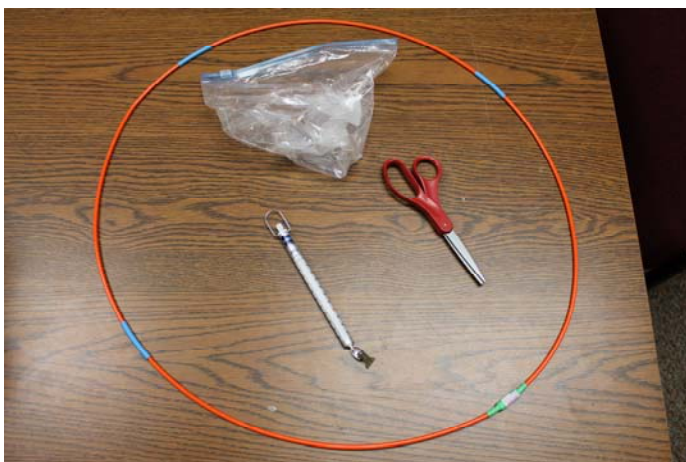
A scale, hoop, scissors, and bags are tools needed for collecting samples with the clip and weigh method.
