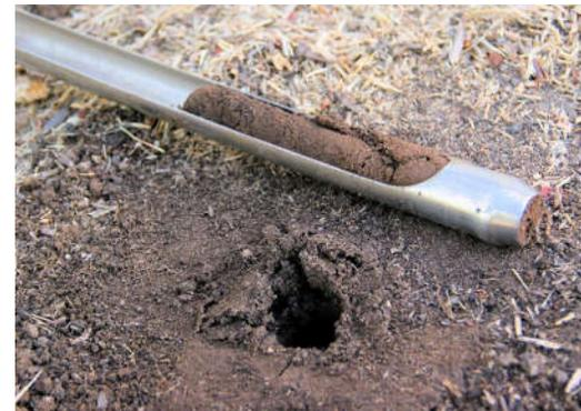
Figure 1: Using a soil probe to obtain a soil core sample.
